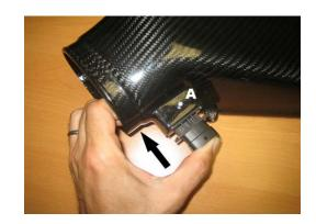
**TIP:** A drop of glue (included in the engine cover kit) on the threads of the Allen screw will prevent it from loosening in the future.
