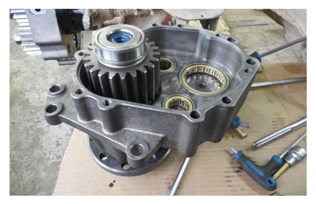
Now the front housing with the lower gear is ready for mounting. Carefully apply sealant all around.
