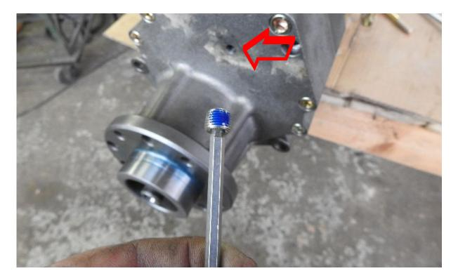
Mount the plug in the center. Apply thread locker.
