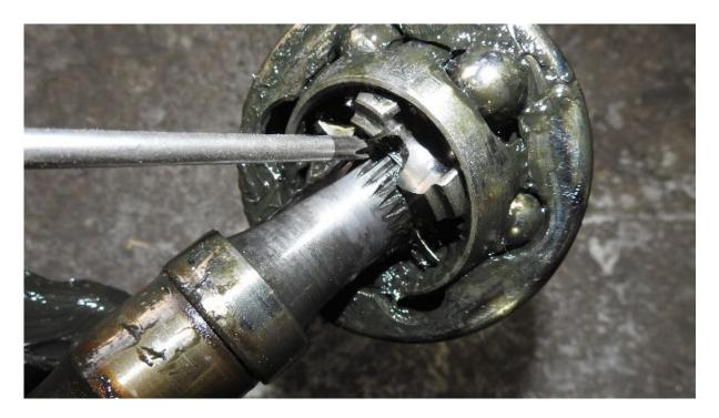
Locate the snap ring and remove the CV joint. Sometimes the CV will not come off easily. In this case you have to cut the CV apart.
