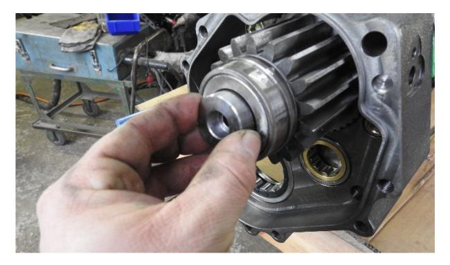
Mont the upper gear and fix the axle shaft with the provided shim and bolt.
