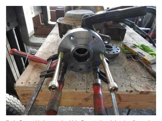
Fix the flange with clamps and weld the flange to the axle housing all around.
