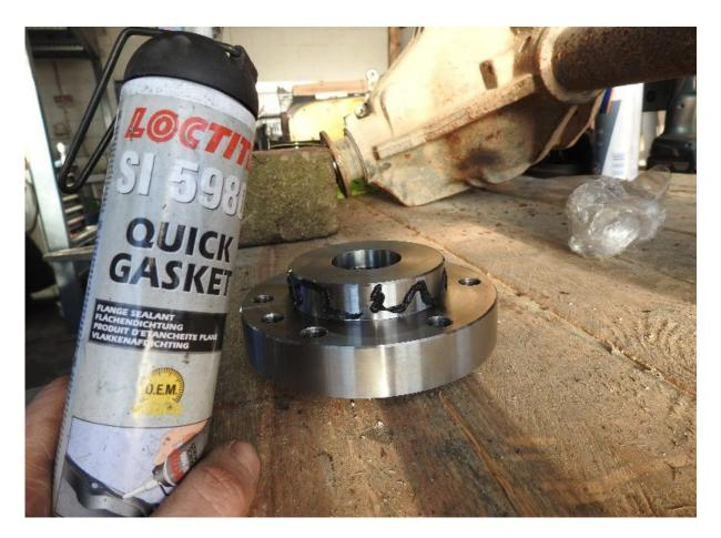
Take the adapter, apply some silicon sealant. Notice: The adapter shown is for disc brake. The adapter for drum brakes looks different.
