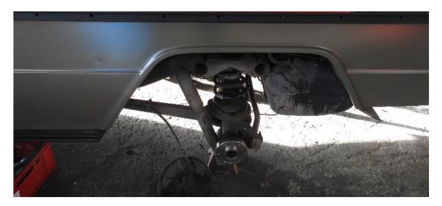
Level the car with jacks under the axle. The axle has to be in ride height.
