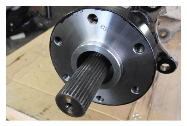
Stick the axle shaft in to the housing. The axle shaft should stick out not more than 65mm.
