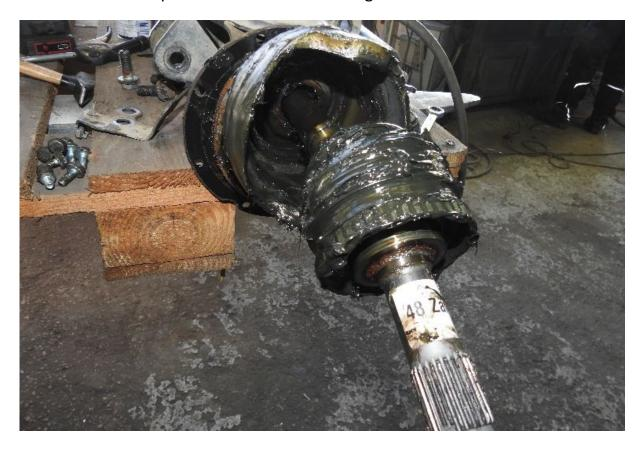
Next remove the steering knuckle and pull the axle shaft.
