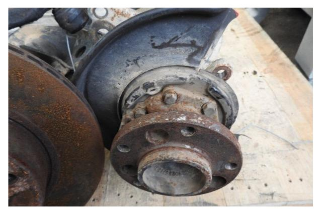
Rear axle: Remove the brake parts and pull the axle shaft out.
