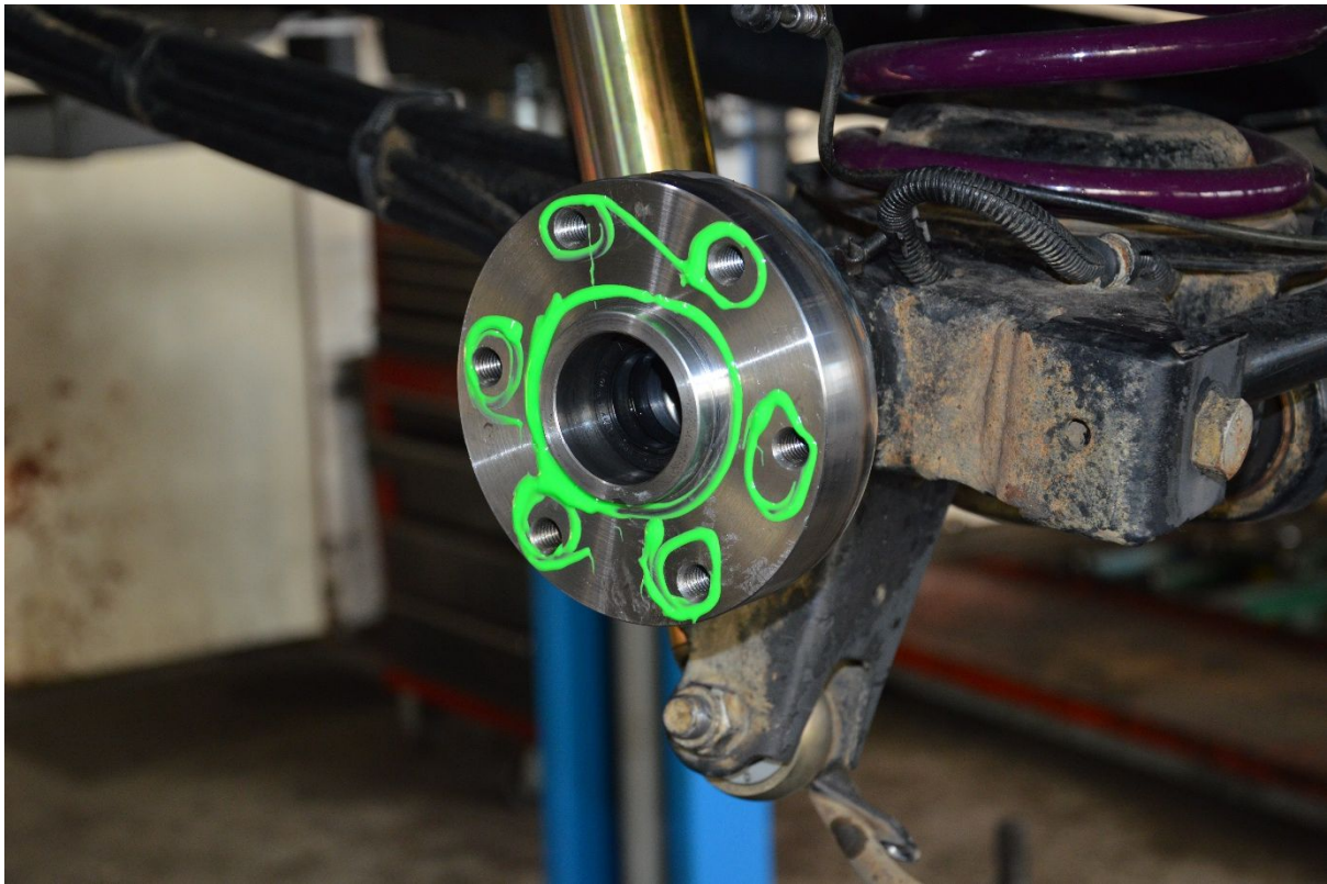
Apply sealant on the flange
