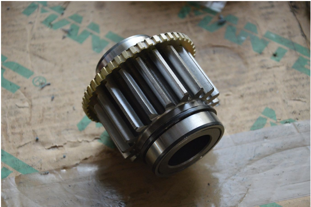
This is the upper gear with the ABS ring installed
