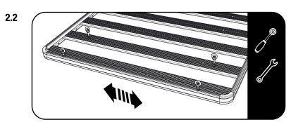
Set the final position with a MaxTrax Resting on the Bolts and fully Tighten.
