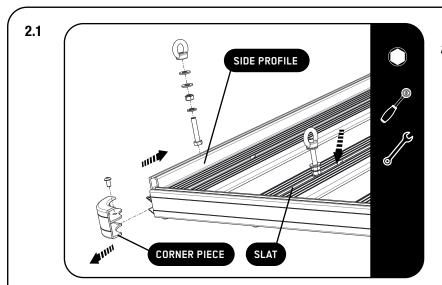
Remove the Corner Piece and feed the two shorter Bolts (see Figure 1.1) into the Channel of the Side Profile and loosely tighten.
