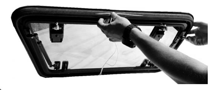
(  ${\bf D}$  ) Place the Gulling Door into position, making sure the the String is to the inside of the vehicle as shown.
