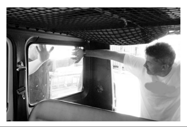
( **B** ) Remove the rubber seal from the original window and fit it to your Gullwing Window as shown. Ensure that the flat side of the rubber is facing the outside of the Gullwing Window.
