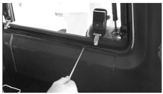
( **F** ) Using the nut and bolt system as indicated by the arrow, adjust the door lock tension on the frame to align the door appropriately.
