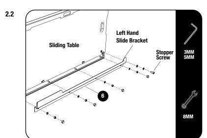
Fit and secure the left hand slide bracket (Item6) with the fasteners you removed in Step 2.1.
