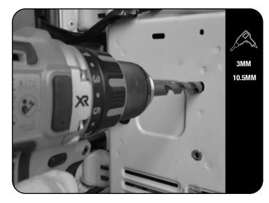
Drill a 3mm pilot hole, using light pressure and taking care only to drill through the interior panel.
