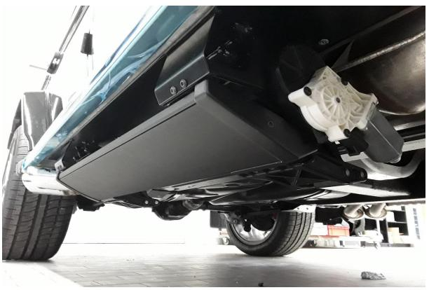
Please check that the electric side step are fully functional. When the door is opened, the footboard should extend and the LED lights should light up. If you have installed the only front door running boards, the side step will only drive out when the driver's door or just the front passenger door is opened. If you have installed the front and rear door version, the side step must extend when the driver's door or the rear door is opened. The same applies to the passenger side.
