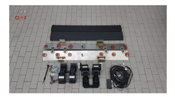
Attach bracket no. 1 with the supplied screws. One rleft side and one rigth side. The screws must be screwed exactly at the positions shown (because they are different in length) and tightened together with the bracket. 25 - 30 torque are sufficient.
