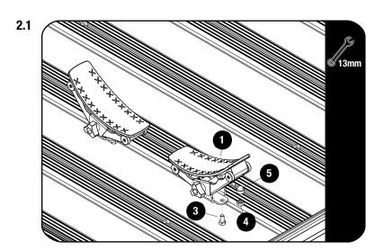
Decide where on your roof rack you would like to place the Kayak Cradle Brackets (Item 1). Work out the correct spacing between the two carriers according to the length of the kayak you are carrying.
