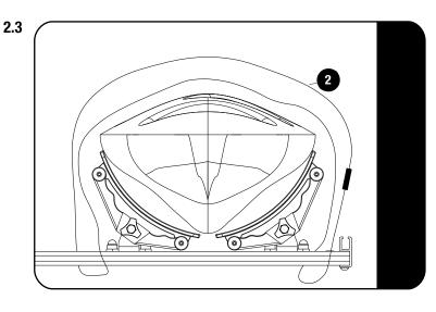
Secure the Kayak / Canoe using the Tie Down Straps supplied (Item 2) by looping them around the roof racks slats.
