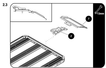
To fit onto a Slimline II Rack, hook the assembled bracket from step 2.1 onto the side profile between two slats.
