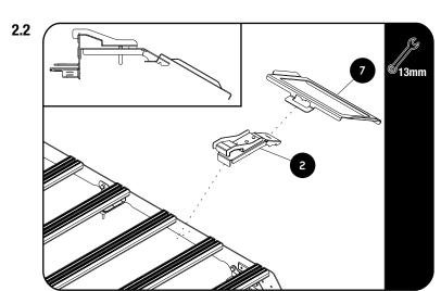
To fit onto a Slimsport Rack, hook the assembled bracket from step 2.1 onto the foot rail between two slats.
