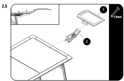
To fit onto a TBRA015 and TBRA019 Table, turn the assembled bracket from step 2.1,180 degrees and loosen the M8 Eye Nut, to allow for clamping onto the Table. Hook the Top Mounting Bracket onto the angled support profile on the underside of the table.
