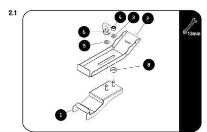
Position the Top Mounting Bracket (Item 1) on a flat surface, with the studs facing up.
