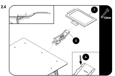
To fit onto a TBRA035 Table, turn the assembled bracket from step 2.1,180 degrees and loosen the M8 Eye Nut, to allow for clamping onto the Table. Hook the Top Mounting Bracket onto the angled support profile on the underside of the table.
