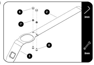
Assemble the Front and Rear Straps using M5 x 10 Button Head Bolts and M5 Nyloc Nuts (Items 7 & 8) as shown.
