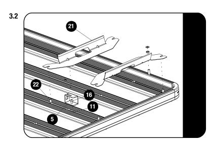
Assemble the M8 x 12 Button Head and M8 Thin Nut (Items 11 & 16) to the Rear Mount Bracket (Item 5).
