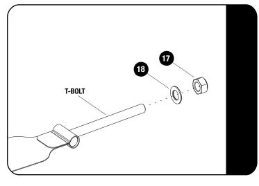
Loosely fit the M6 Nyloc Nut and M6 x 12 x 1 Flat Washer (Items 17 & 18) to the T-Bolts at the en for the Rear Strap as shown.
